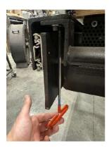
4. Use the same ¼" allen wrench to remove the aluminum table shoulder bolts and springs from the assembly. Only remove the shoulder bolts and springs from the side you are replacing the slide on. \*(Take a picture with your phone before removing hardware for a future reference)
