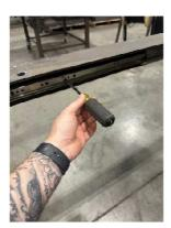
6. Next remove the  $10-32 \times 1/2$ " phillips screws that are used to attach the slide to the frame of the machine. Do this by moving the slide in and out to can access to the heads of the screws through holes in the slide.
