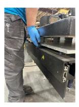
2. Slide a ¾" thick shim/wood block between the bottom of the aluminum table plate and the top of the black tubing of the lift plate.
